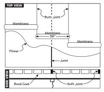
perimeter tape at room perimeter. Soft joints in tile patterns are required as per TCNA Handbook method EJ171.
