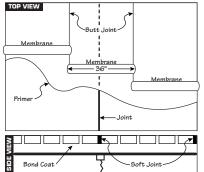
have a minimum 1/8" gap at all floor to wall transitions. Apply an acoustical sealant or sound perimeter tape at room perimeter. Soft joints in tile patterns are required as per TCNA Handbook method EJ171.
